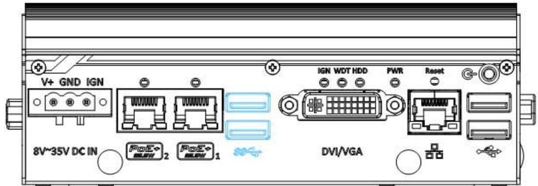
The system offers two USB 3.0 (SuperSpeed USB) ports on its front panel. They are implemented by native xHCI (eXtensible Host Controller Interface) controller in Atom E3950 SoC and are backward compatible with USB 2.0, USB 1.1 and USB 1.0 devices. Legacy USB support is also provided so you can use USB keyboard/mouse in DOS environment while xHCI driver is supported natively in Windows 10.
