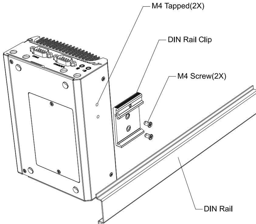
2. To install the DIN rail clip onto the DIN rail, you must come over the top of the DIN rail, tilting, overlap the top clip edge of the DIN rail clip onto the DIN rail first, and then firmly press the bottom-front of the enclosure to clip the bottom edge of the mount plate.
