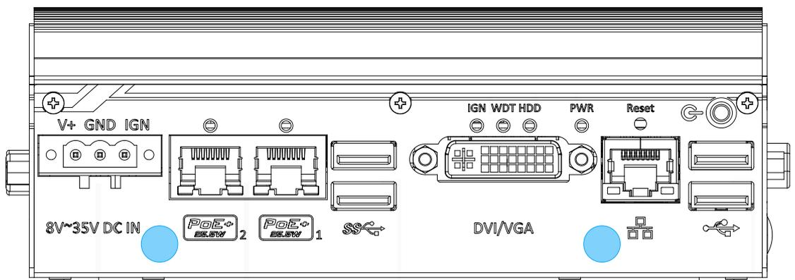
The system offers two SMA antenna openings on the front panel reserved for SMA antenna installations. Users can take advantage of these two openings when installing mini-PCIe module for wireless communication reception such as 3G, 4G, GPS or WiFi.
