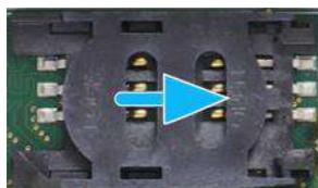
**Push towards the middle of the MezIO™ module to release the slot**
