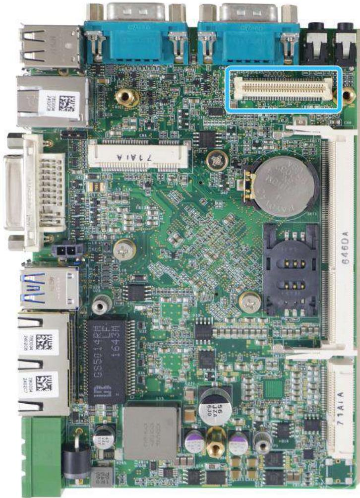
MezIO™ is an innovative interface designed for integrating application-oriented I/O functions into an embedded system. It offers computer signals, power rails and control signals via a high-speed connector. MezIO™ is also mechanically reliable benefited from its 3-point mounted mezzanine structure. A MezIO™ module can leverage these signals to implement comprehensive I/O functions.
