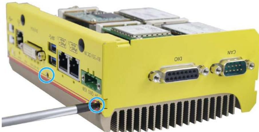
3. Gently slide the L-shaped enclosure panel back into place.
