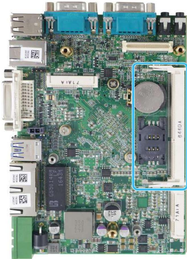
The system has an internal SO-DIMM slot supporting DDR3L-1866 memory module up to 8GB in capacity. The L in DDR3”L”-1866 denotes Low Voltage (1.35V) type SO-DIMM memory modules.
