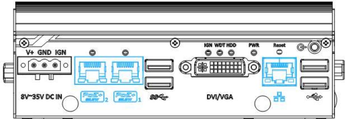
The system offers three Gigabit Ethernet ports using Intel® I210 GbE controller. From top to bottom, they are port #3, #1 and #2. When plugged in and connected via the Ethernet cable, the LEDs on the RJ45 connector indicate connection status and speed.
