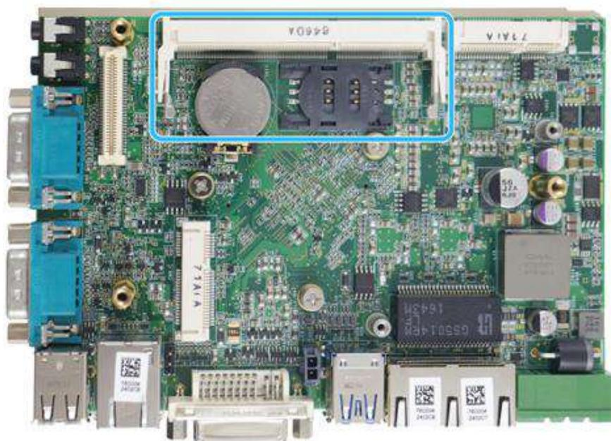
4. **To install**, insert the gold finger end of the SO-DIMM on a 45 degree angle into the slot and gently push the SO-DIMM down until it clips-in.
