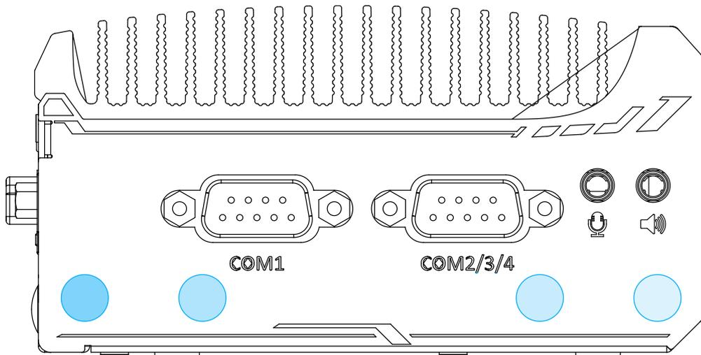
The system offers four SMA antenna openings reserved for SMA antenna installations. Users can take advantage of these two openings when installing mini-PCIe module for wireless communication reception such as 3G, 4G, GPS or WiFi.
