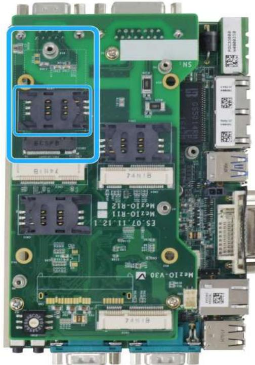
3. To insert a SIM card, push and flip the slide-and-clamp slot towards the center of the MezIO™ module.
