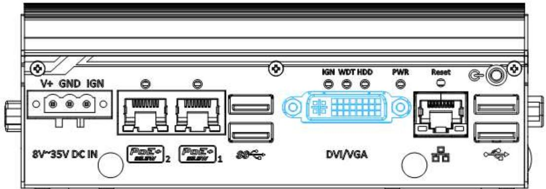
The system features a DVI-I connector on its front panel that is also compatible with VGA signals. The DVI and VGA outputs are directly driven by integrated Intel HD graphics engine and support up to 1920 x 1200 resolution.
