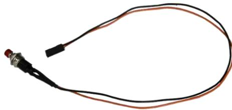
2. Connect the non-latched switch to the **pin#2** and **pin#3** of the on-board 1x3 pins, 2.0mm pitch pin header (polarity is negligible). Press the button on the switch to turn on the system.
