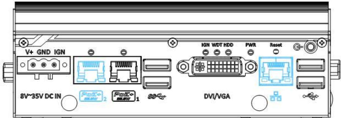
The Power over Ethernet (PoE) port supply power and data on a standard CAT-5/CAT-6 Ethernet cable. Acting as a PSE (Power Sourcing Equipment), compliant with IEEE 802.3at, each port delivers up to 25W to a Powered Device (PD). PoE automatically detects and determine if the connected device is PoE PD or not before supplying power, making it compatible with standard Ethernet devices as well.
