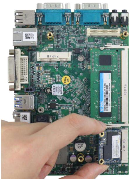
4. Gently press the card down and secure with a screw.
