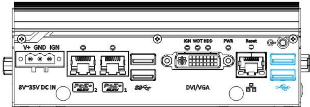
The USB2.0 ports are implemented via native xHCI (eXtensible Host Controller Interface) controller in Atom E3950 is backward compatible with USB 1.1 and USB 1.0 devices. Legacy USB support is also provided so you can use USB keyboard/mouse in DOS environment.
