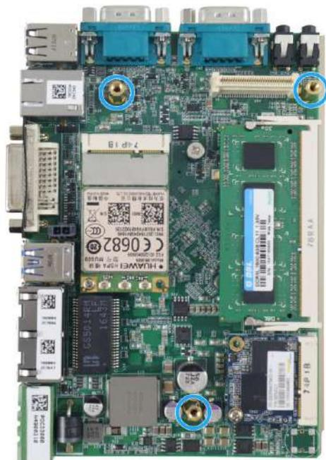
3. Gently lower the module onto the mainboard. The MezIO™ port should engage if the three (3) standoffs and screw holes meet. Then secure the MezIO™ module to the hex bolts with three (3) P-head screws.
