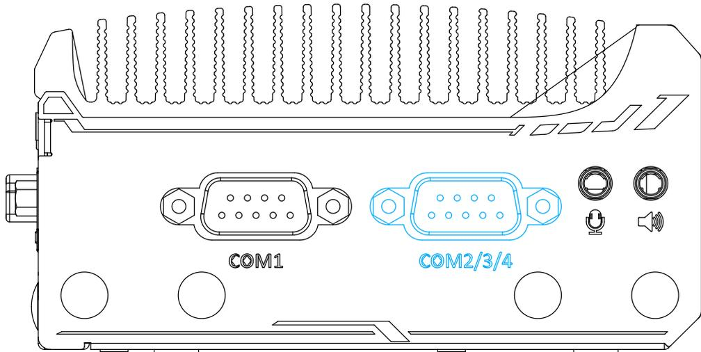
Implemented using industrial-grade ITE8786 Super IO chip (-40 to 85°C) and provide up to 921600 bps baud rate, the second D-Sub male connector (COM2/ 3/ 4) can be configured in BIOS as single RS-422/ 485 port (COM2) or three 3-wire RS-232 ports (COM2/COM3/COM4). Please refer to [COM2/ 3/ 4 Port Configuration](#) for configuring operation mode. An optional 1-to-3 Y-cable is available to connect three RS-232 devices.
