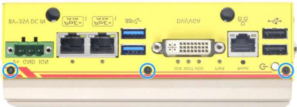
3. Remove the two (2) screws at the rear.
