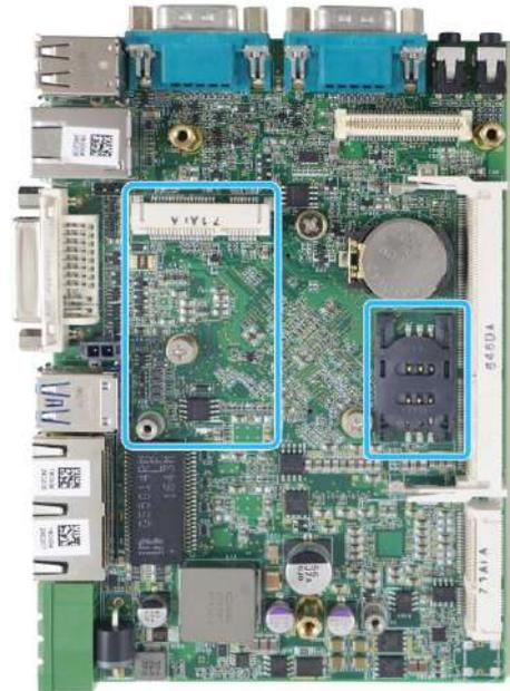
mini-PCIe/ SIM slot on the mainboard
