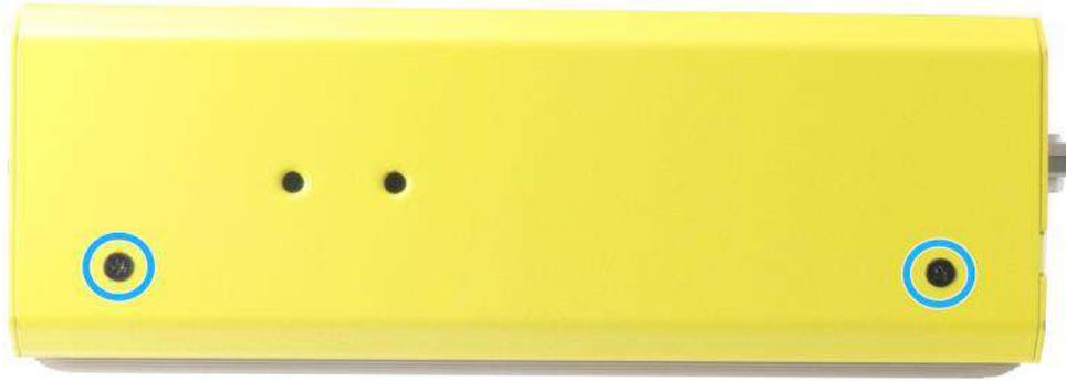
4. Gently slide out the L-shaped panel and remove the screw that holds the DIO/ CAN port panel. Remove the DIO/ CAN port panel.
