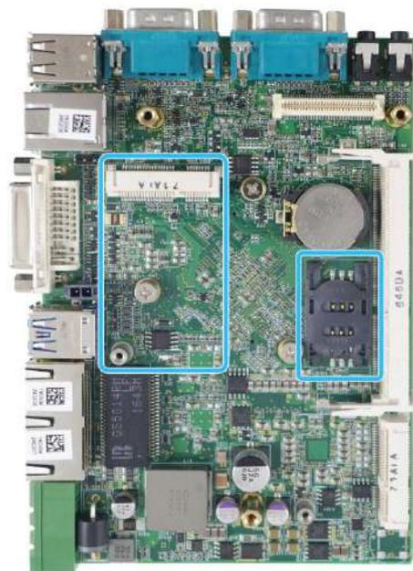
**mini-PCle/ SIM slot on the mainboard**
