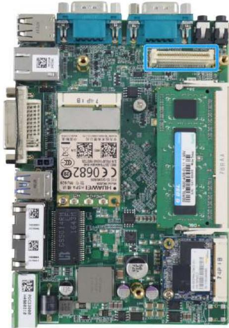
2. The stand-off hex bolts can be located on the mainboard. Place the MeziO™ module on top of the mainboard, match the three hex bolts and the MeziO™ connector should meet.
