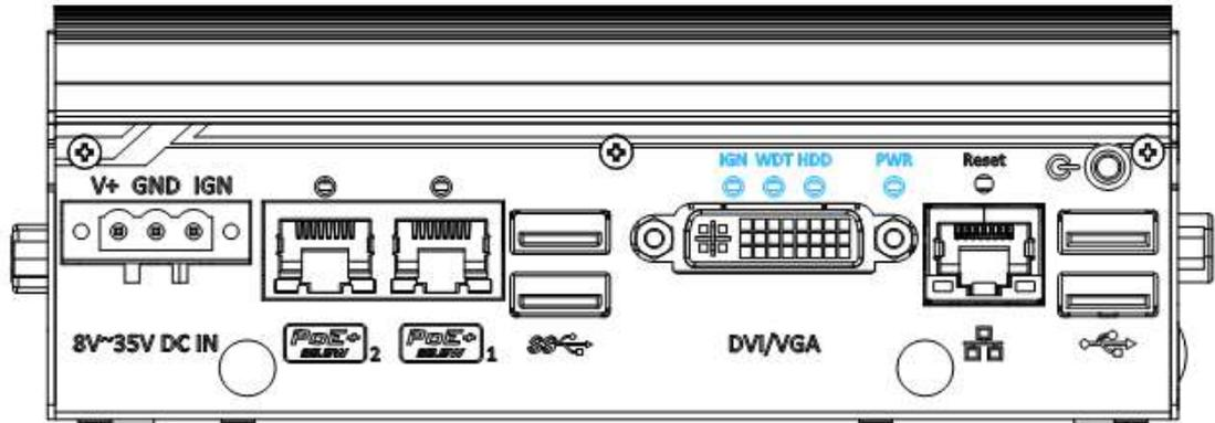
There are four LED indicators on the front panel: PWR, HDD, WDT and IGN. The descriptions of these four LEDs are listed in the following table.
