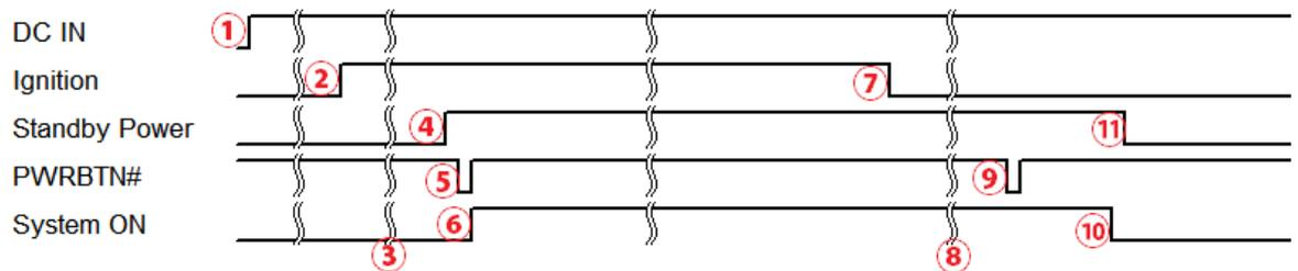
1. When DC power is supplied to the system, MCU starts to periodically detect ignition signal. Note that only MCU is working at this moment and the overall power consumption is less than 2 mW.
