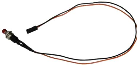
2. Connect the latched switch to the **pin#1** and **pin#2** of the on-board 1x3 pins, 2.0mm pitch pin header (polarity is negligible).
