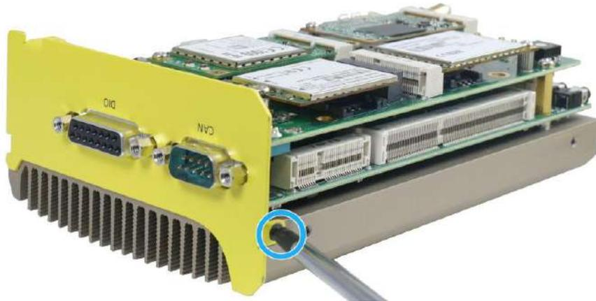
2. Install the front panel and secure it with two (2) screws indicated in the illustration below.
