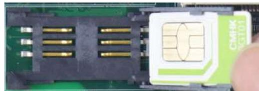
**Flip towards the middle of the MezIO™ module to open the slot and insert the SIM card**
