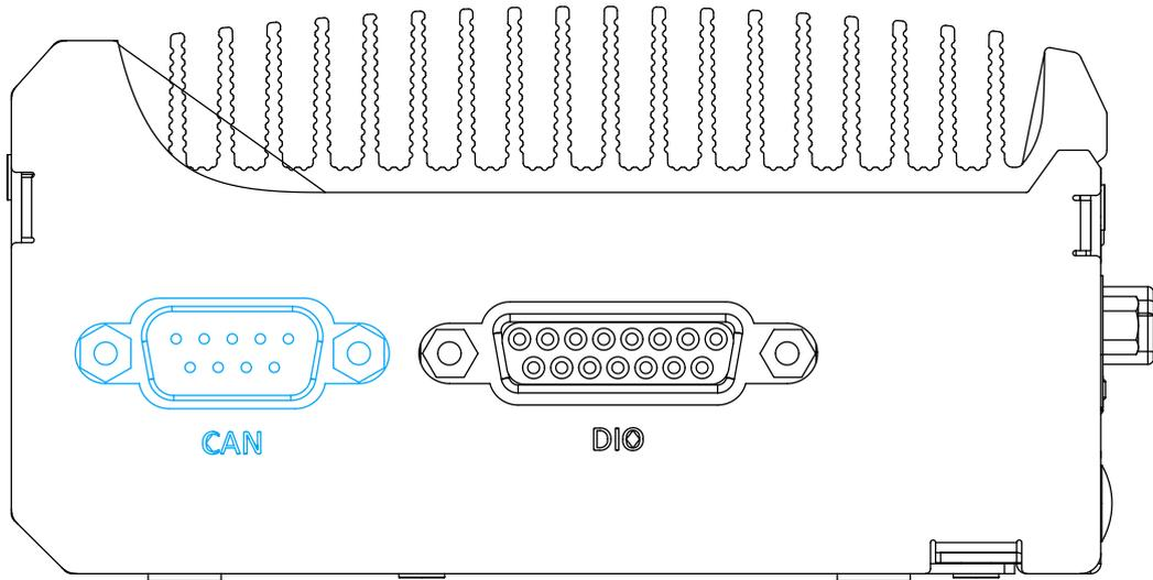
CAN bus is a robust industrial bus with a pair of differential signals and is commonly used in various industrial and in-vehicles applications. The system is equipped with a CAN bus DB9 port that is compatible with both industrial and in-vehicle applications. The CAN bus port supports CAN2.0A and CAN2.0B up to 1Mbps.
