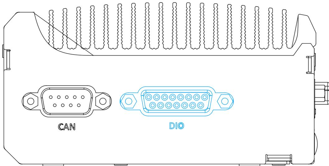
The system provides 4x isolated digital input channels and 4x isolated digital output channels. The DIO functions support polling mode I/O access and DI change-of-state interrupt. Please refer to [Watchdog Timer & Isolated DIO](#) for information on wiring and programming the isolated DIO channels.
