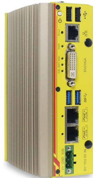
External connection wise, POC-351VTC has three Gigabit Ethernet ports (two are 802.3at Gigabit PoE+ ports), two USB3.0 ports, two USB2.0 ports, one DVI-I connector for VGA + DVI dual video output, four COM ports, CAN bus, four isolated DI and four isolated DO. The rich assortment of I/O ports allow easy data communication with other devices.
