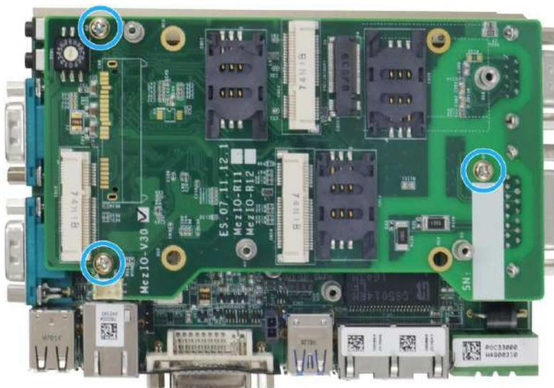
4. **To install**, insert mini-PCIe module's gold finger on a 45 degree angle into the socket, gently press the module down and secure it with a screw.
