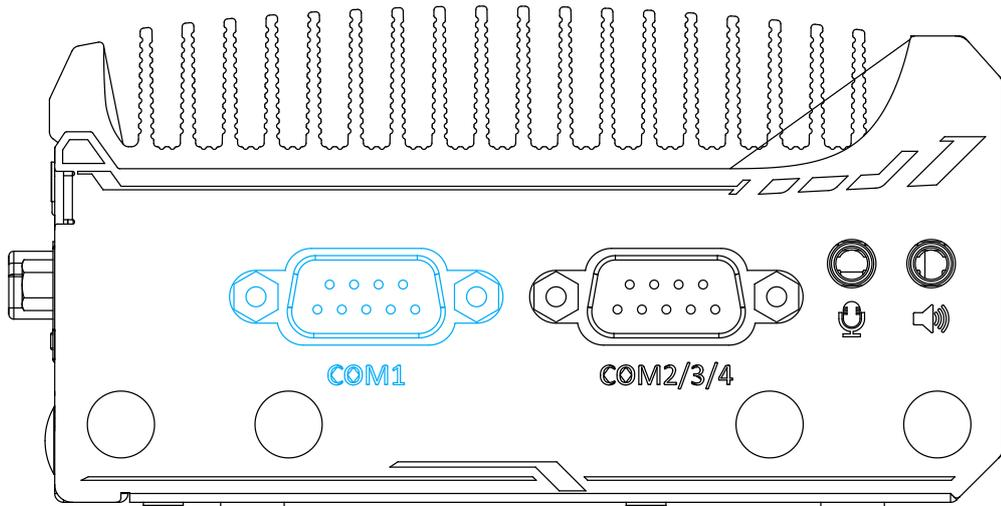
Implemented using industrial-grade ITE8786 Super IO chip (-40 to 85°C) and provide up to 921600 bps baud rate, COM1 is a software-configurable RS-232/422/485 port via 9-pin D-Sub male connector. The operation mode, slew rate and termination of COM1 can be set in BIOS setup utility. The following table describes the pin definition of COM ports.
