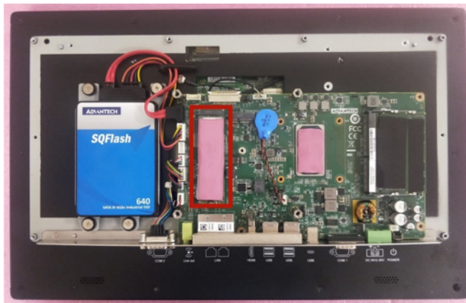
Figure 2.13 Affix the Thermal Pad to the M.2
