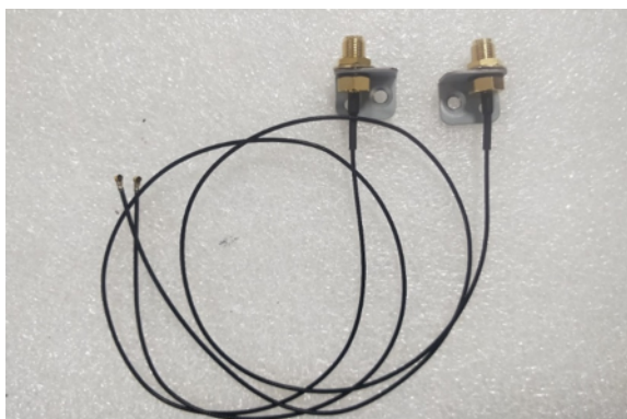
Figure 2.14 Assemble the Brackets to the Antenna Cables
