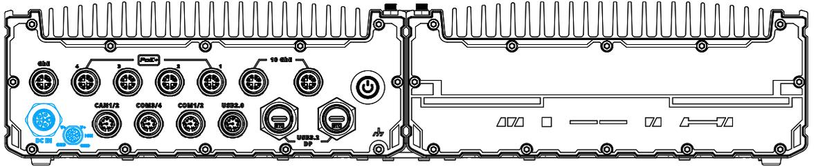
The system accepts a wide range of DC power input from 8V to 48V with reverse polarity protection via a M12 L-coded connector. The M12 L-coded connectors offer COTS availability and ultra-rugged connection reliability when wiring DC power.
