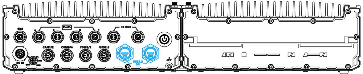
The system's USB 3.2 Gen1x1 type-C port offers up to 5Gbps of data transfer bandwidth, and is implemented via the native xHCI (eXtensible Host Controller Interface) controller. The port is backward compatible with USB3.2 Gen.1 USB 2.0, USB 1.1 and USB 1.0 devices via a USB hub (not included) to connect to external devices.
