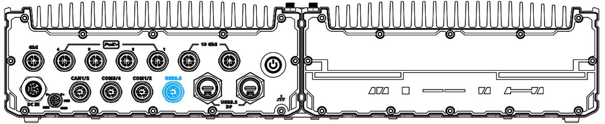
The USB2.0 ports are implemented via native xHCI (eXtensible Host Controller Interface) controller and are backward compatible with USB 1.1 and USB 1.0 devices. Legacy USB support is also provided so you can use USB keyboard/mouse in DOS environment.
