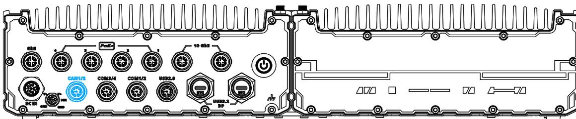
CAN bus is a robust industrial bus with a pair of differential signals and is commonly used in various industrial and in-vehicles applications. The CAN bus port supports CAN2.0A and CAN2.0B up to 1Mbps.
