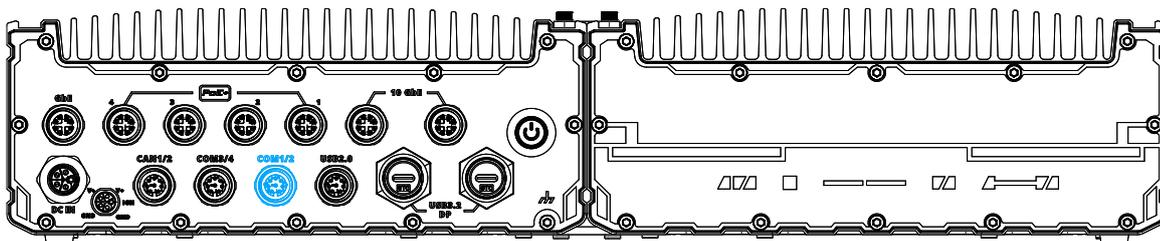
The system provides two isolated COM ports via an M12 A-coded connector for communicating with external devices. COM 1 and 2 ports are 3-wire RS-232 specifications and provide up to 115200 bps baud rate.
