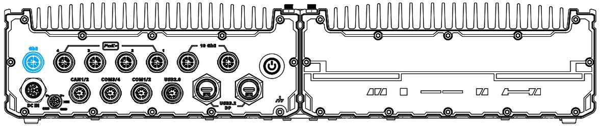
The system offers one Gb Ethernet port implemented Intel i219. It supports Wake on LAN and is also compatible with Intel® AMT (Active Management Technology) to support advanced features such as remote SOL desktop and remote on/ off control.
