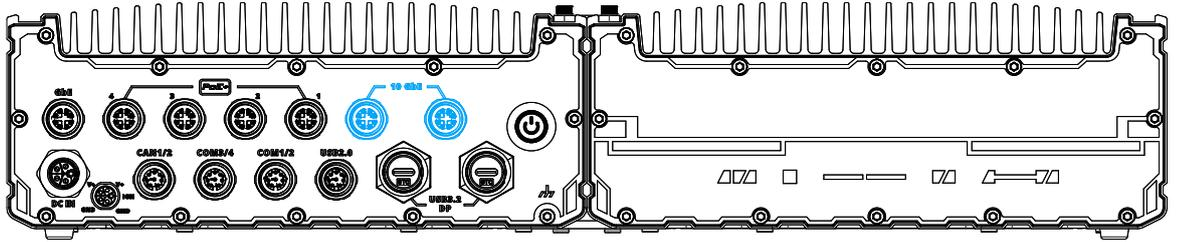
The system offers two 10Gb Ethernet ports supporting Wake-on-LAN via M12 X-coded connector implemented using Intel® X550AT controller on the front panel. The port is backwards compatible with 5Gb, 2.5Gb, and Gb Ethernet connections.
